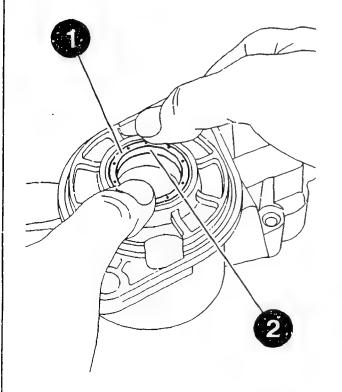
COMPONENT CHECKING AND REPAIR Checking drive-end shield (version with bushing) Installing radial lip-type oil seal contd.: Use small cape chisel to caulk driveend shield at four locations (1) (offset by 90 in each case) to ensure tight fit of radial lip-type oil seal. Take care not to damage machined seat of radial lip-type oil seal. Remove surplus grease after installation.
